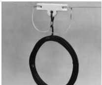
Figure 20.24 — RF choke formed by coiling the feed line at the point of connection to the antenna. The inductance of the choke isolates the antenna from the outer surface of the feed line.
