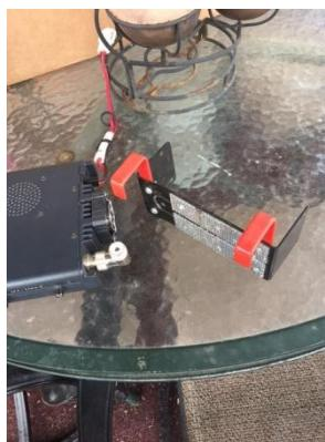
Fourth, screw the brackets to the radio mounting bracket and attach to the cup holder. Connect the antenna and power and you are good to go.
