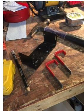
First, cut off the closed end of the bracket to make two 6 ½ "flat pieces of metal. Second, using the mounting bracket for the radio measure and drill 2 mounting holes for each bracket. The can be either the top or bottom of the radio, your choice. Third, measure the cup holder lip size, using a vice make two bends in the bracket with your desired opening. Do for the other one.
