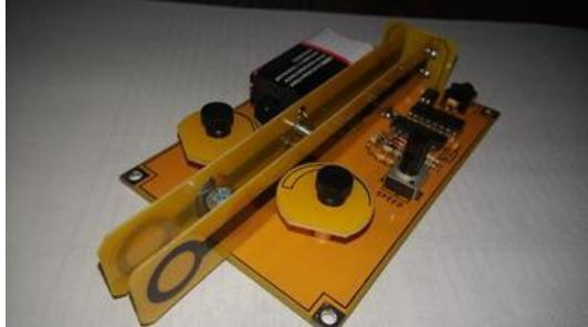
The Cric-Key is a simple CW keyer with paddle, well suited for not only use at home, but in the field as well. This kit is designed to complement 4SQRP's popular CRICKET series of QRP transceivers with a useful and easy-to build keyer circuit. High quality, double sided printed circuit board construction is used, with solder mask and silk screened component reference designators. All components are
