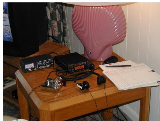
The rig consists of: Yaesu FT 857, 100 Watt, 160-70 cm transceiver, SEC 1223 Power supply, MFJ 904h antenna tuner, MFJ iambic paddle (packed under tuner), Antenna base 3/8" x 24, all necessary cables, coax and counterpoise, etc. Case size: 16" L, 13" W, 13" H.
