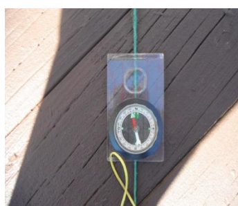
Compass indicating difference between magnetic and true North
