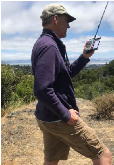
Wayne Burdick, N6KR, using a KH1 while operating solo during 2024 ARRL Field Day. He operated on 20- and 15-meter CW, using an "invisible" #26 AWG trailing ground wire. [Griffin Svec-Burdick, photo]
